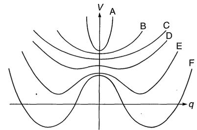
**Fig. 1.** Potential  $V$  as a function of particle position  $q$  changing with time. The potential starts with a single minimum (curve A), ends up in a deeply bistable state (curve F), and then returns to the single minimum. The relative vertical displacement of curves is selected for clarity and has no significance.
