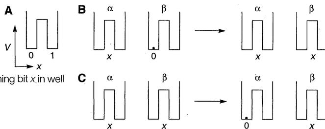
**Fig. 7.** (A) Barrier as a function of the positions of the two particles involved before time modulation begins. (B) Shaded region has reduced barrier during copying of  $\alpha$  to  $\beta$ . The barrier in the receiving  $\beta$  well is lowered if and only if the particle in the controlling  $\alpha$  well is in the 1 state. (C) Shaded region has reduced barrier during resetting for particle in well  $\alpha$ .
