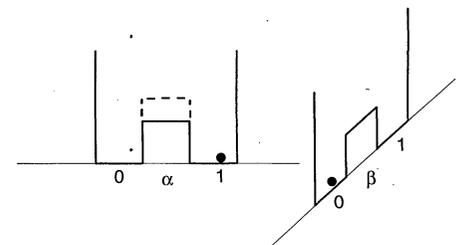
**Fig. 8.** Controlling  $\alpha$  well is perpendicular to controlled  $\beta$  well. The position of  $\alpha$  controls the barrier of  $\beta$ . The  $\alpha$  barrier can be increased temporarily to lock the  $\alpha$  particle firmly in its position.
