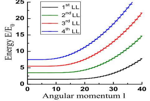
FIG. 2: The energy dispersion of the first four Landau levels *v.s.*  $l = j - \frac{1}{2}$ . Open boundary condition is used for a ball with the radius  $R_0/l_G = 8$ . The edge states correspond to those with large values of  $l$  and develop linear dispersions with  $l$ . The most probable radius of the LLL state with  $l$  is  $r = l_G\sqrt{l}$ .
