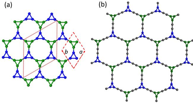
FIG. 1. Atomic structure of (a) kagome graphene, where the primitive unit cell is shown by the dashed red line. Blue and green triangle rings of atoms are two sublattices of the system. Dotted brown line shows a  $\sqrt{3} \times \sqrt{3}$  supercell as a result of Wigner crystallization. (b) Kagome graphyne, where the triangular rings are linked by acetylenic carbon linkers.
