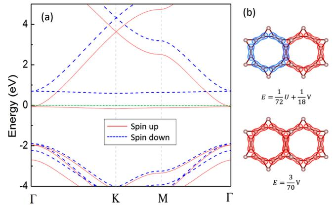
FIG. 3. Flat-band ferromagnetism. (a) DFT band structure of kagome graphene after one-hole doping to result in a ferromagnetic ground state. The green dotted line shows the Fermi level. (b) Wave functions of the localized states in the simplified model [cf. Eq. (1)] with calculated energies. The touching of two localized states with opposite spins would cost more energy than that with the same spin. This energy cost is the origin for the global ferromagnetism seen here.
