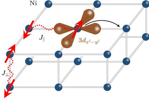
**Fig. 1.** Schematic diagram for the effective single  $3d_{x^2-y^2}$  orbital bilayer  $t$ - $J_{\parallel}$ - $J_{\perp}$  model. Each layer is comprised by a conventional intra-layer  $t$ - $J_{\parallel}$  model, while the two layers interact through an inter-layer spin exchange  $J_{\perp}$ .
