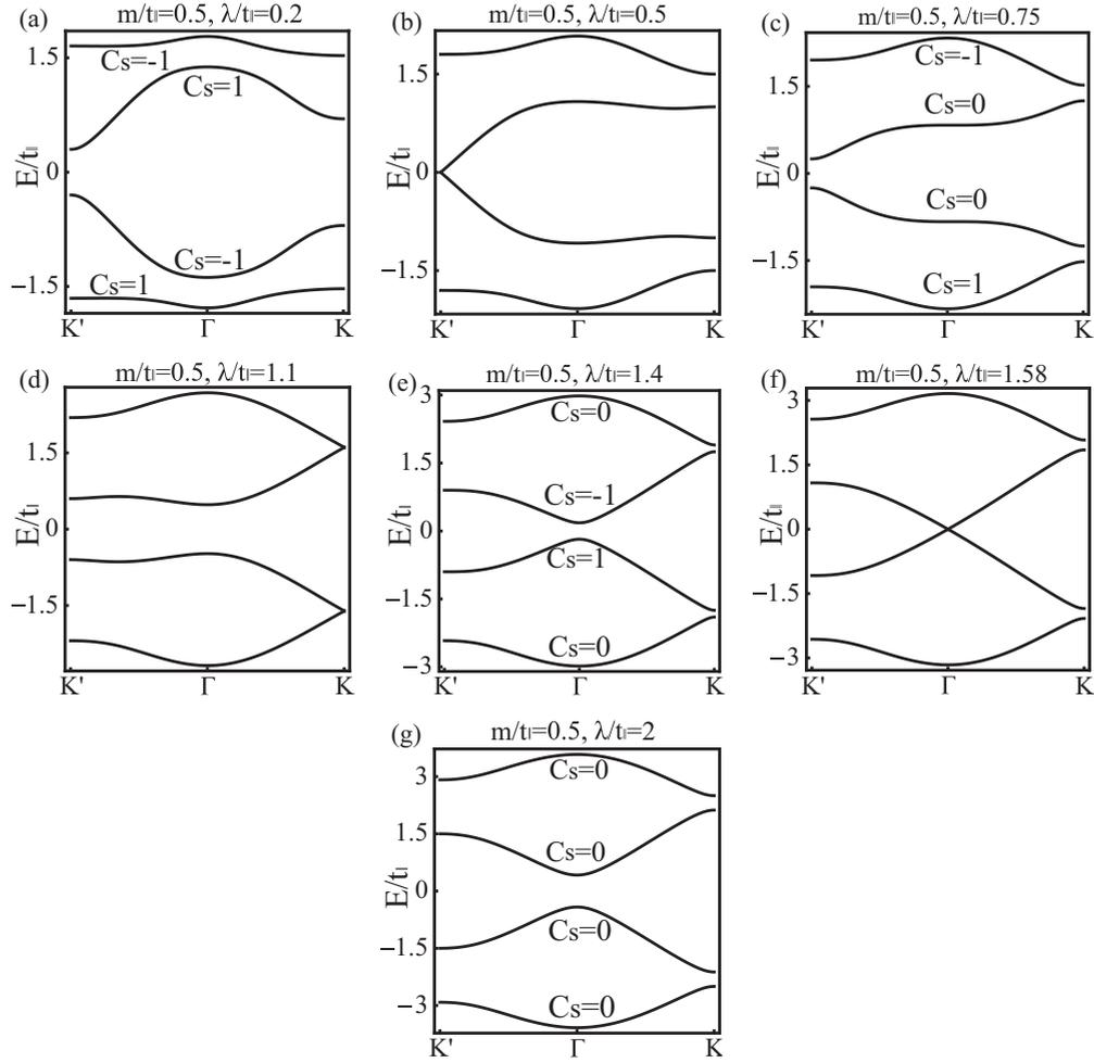
FIG. 3. The same plot as in Fig. 2 but for the evolution with fixed  $m/t_{\parallel} = 0.5$  and increasing  $\lambda$  from 0.2 (a) to 2 (g), which passes phases  $A_1$ ,  $B_1$ , and  $B_2$  and  $C_1$ . Gaps are closed at  $K'$ ,  $K$ , and  $\Gamma$  points in (b), (d), and (f), respectively.
