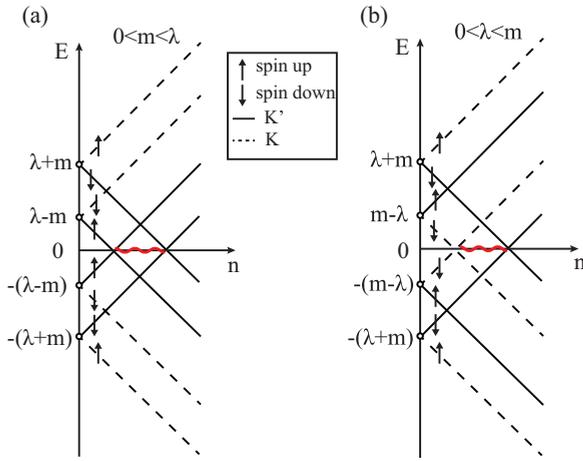
FIG. 6. (Color online) Diagrams of the energy level crossing with increasing antiferromagnetic exchange field strength  $n$  for two parameter regimes (a)  $0 < m < \lambda$  and (b)  $0 < \lambda < m$ . Red wavy lines indicate the range of  $n$  for the system to be in a QAH phase ( $|\lambda - m| < n < \lambda + m$ ).
