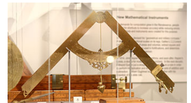
Galileo's geometrical and military compass , thought to have been made c. 1604 by his personal instrument-maker Marc'Antonio Mazzoleni
