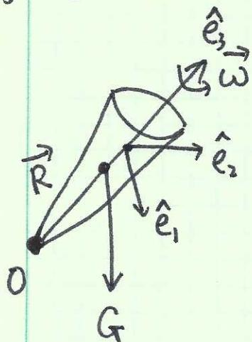
symmetric top spinning in the gravity
