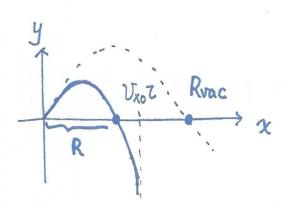
The range on the horizontal direction in the vacuum
