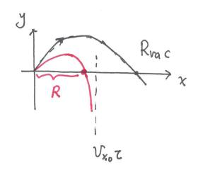
$$R \approx R_{\text{vac}} \left[ 1 - \frac{4}{3} \frac{V_{\text{yo}}}{V_{\text{(00)}}} \right]$$
