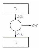
As shown above, two "identical" bodies of constant heat capacity  $C_p$ , originally at temperatures  $T_1$  and  $T_2$ , are used as reservoirs for a Carnot engine operating in infinitesimal reversible cycles. If the bodies remain at constant pressure and undergo no phase changes,
