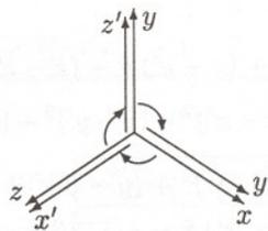
A  $120^\circ$  rotation carries the  $z$  axis into the  $y$  ( $= \bar{z}$ ) axis,  $y$  into  $x$  ( $= \bar{y}$ ), and  $x$  into  $z$  ( $= \bar{x}$ ). So  $\bar{A}_x = A_z$ ,  $\bar{A}_y = A_x$ ,  $\bar{A}_z = A_y$ .
