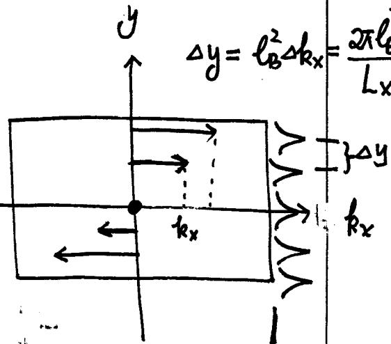
In other words, the  $y$ -axis plays the role of the momentum of the  $x$ -axis. If we only keep the LL states (this is justified in the case of the gap between LLs  $\hbar\omega_c$  is much larger than all the other energy scales that we are interested, i.e. in the limit of  $\hbar\omega_c \rightarrow +\infty$ . This process is called LLL projection).
