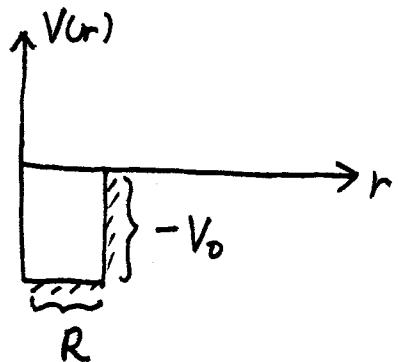
$$\left. \begin{array}{l} \text{at } r < R, \quad u = \sin k_0 r \\ r > R \quad u = A e^{-\beta r} \end{array} \right\} \Rightarrow \left. \begin{array}{l} \frac{u'}{u} \Big|_{r=R} = k_0 \cot k_0 R \\ \frac{u'}{u} \Big|_{r=R} = -\beta e^{-\beta R} \end{array} \right.$$
