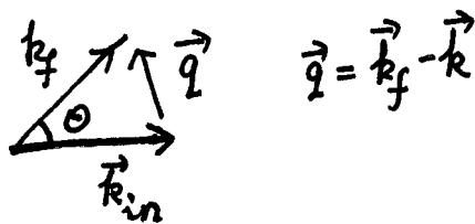
$$\Rightarrow \psi(r) = e^{i\vec{k}_i \cdot \vec{r}} - \frac{e^{ikr}}{r} \frac{m}{2\pi\hbar^2} V(\vec{k}_f - \vec{k}_i) \Rightarrow f(\vec{k}_i, \vec{k}_f) = -\frac{m}{2\pi\hbar^2} V(\vec{k}_f - \vec{k}_i)$$
