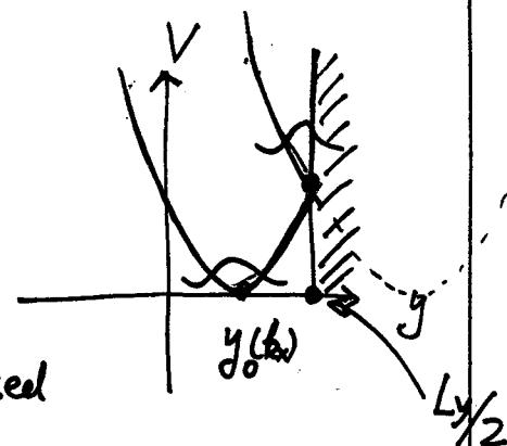
For states  $k_x < \frac{L_y}{2\ell_B^2}$ , its center of  $V_{k_x}(y)$  is away from the boundary, thus it's not affected by the boundary. But as  $k_x > \frac{L_y}{2\ell_B^2}$ , its bottom is cut by the boundary, and thus its energy is pushed up. Even at the classical level, we have
